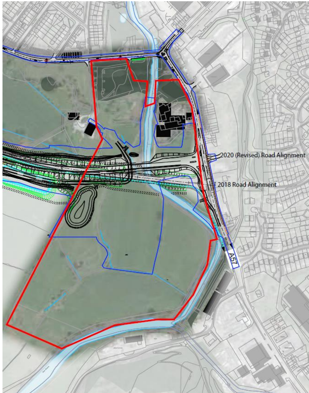
Figure 1: 2018 road alignment vs 2020 road alignment
